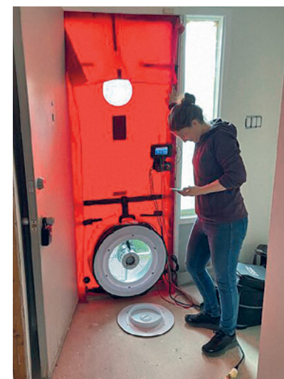
► Testing air tightness
